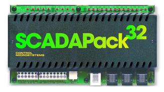
The SCADAPack 32 utilizes the same lower I/O board as the traditional SCADAPack with 8 analog inputs, 20 digital inputs (3 of which can be use as high speed counters for turbine meters), 2 optional analog outputs, and 12 relay outputs. Expansion to over 700 I/O points is possible through the addition of 5000 series modules.
