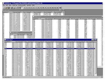
and cmi date in the format yyyy/mm/dd/hh/mm/ss. The number of records that may be logged in a SCADAPack or Micro16 controller will depend on the size of memory available. With the 512K RAM option installed approximately 198,000 words of data may be logged in the controller.
